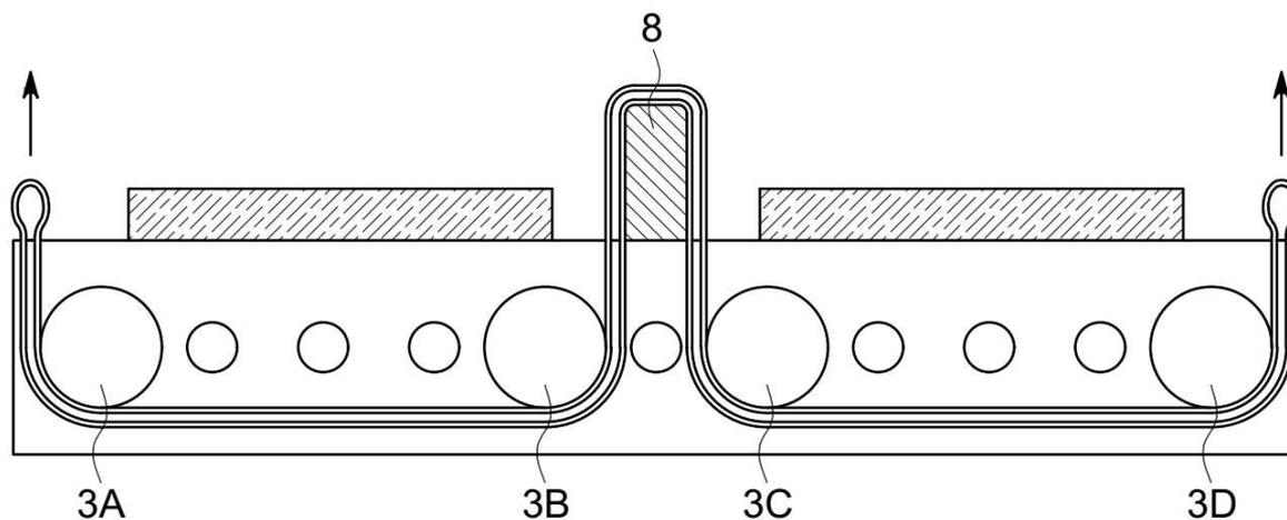
Run a single band around rollers 3A and 3D.
