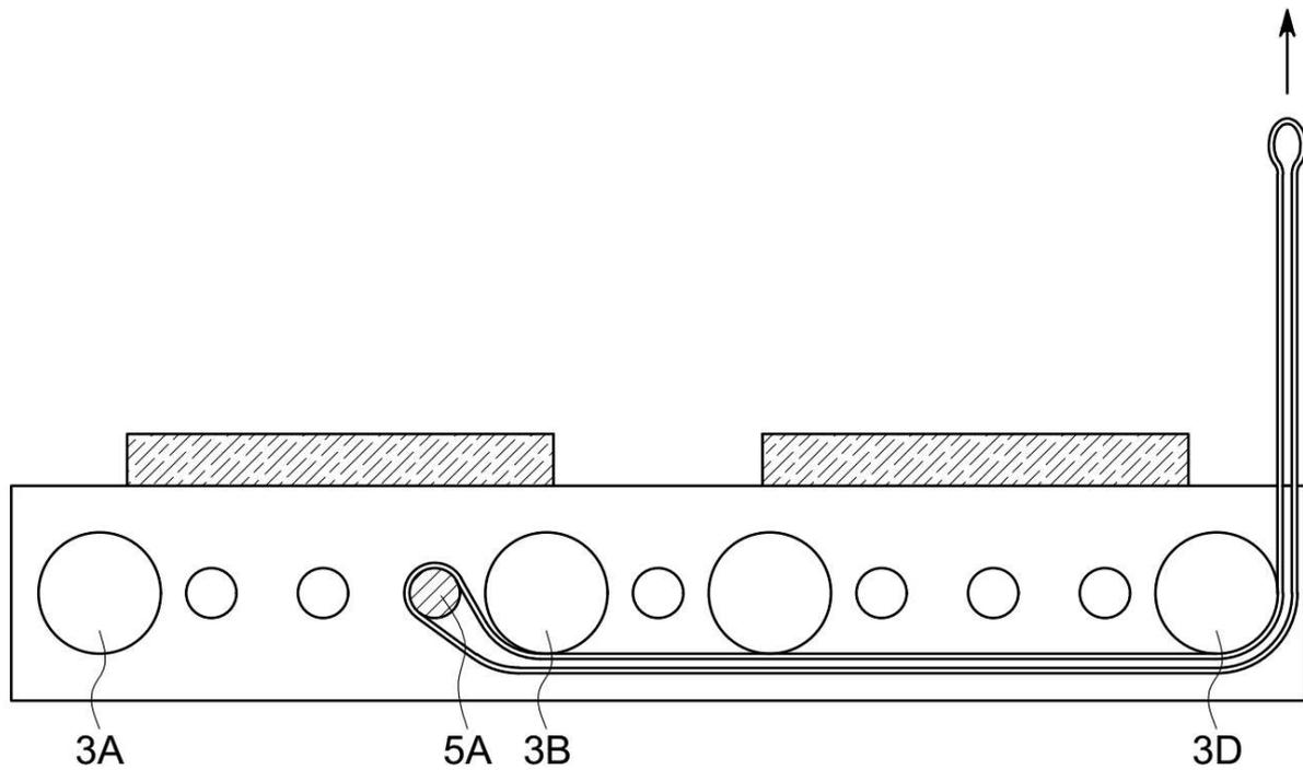
For a high starting point, redirect the band around roller 3D, and hold it in place with pin 5A.
